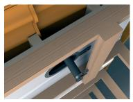
3. Support the pipes under the pass-through so that it carries the weight of the pipes under it.
